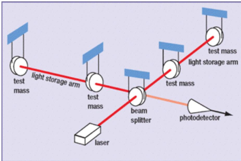
Figure 1: A schematic diagram about inner structure and basic principles of how LIGO works
